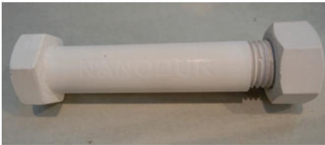
Concrete bolt as a component of a concrete canoe
