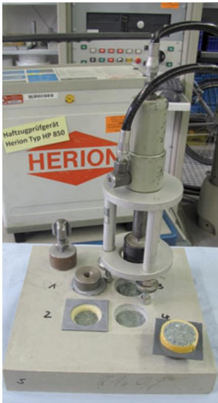
Testing the surface tensile strength
