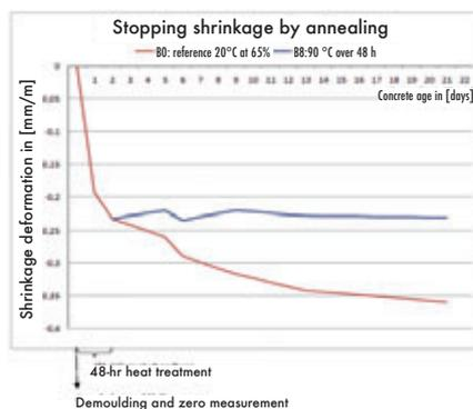
Stopping shrinkage by annealing
