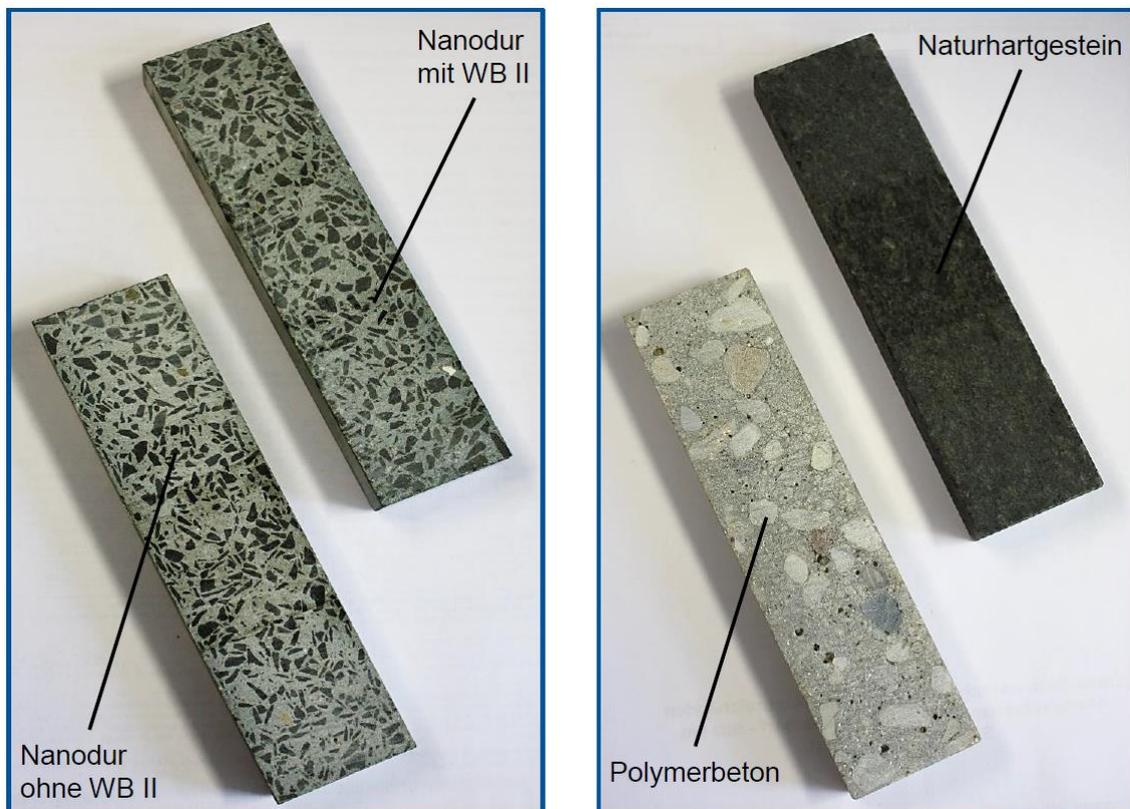
Tested specimens made of Nanodur-concrete, epoxy based mineral cast and natural stone
