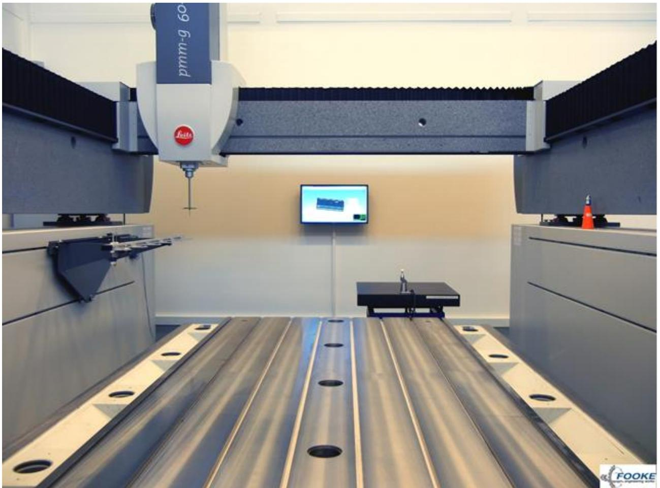
3D-measuring machine made of Granite, test specimen made of Nanodur-Concrete
