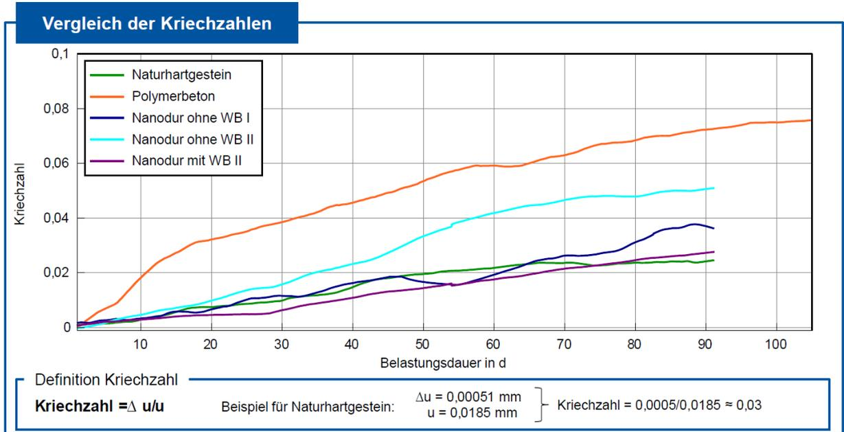
Comparison of characteristic creep values of natural stone (green), various samples of Nanodur-Concrete und epoxy bound mineral cast (red)
